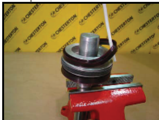
3. Use a non-metallic tool to assist stretching the seal fully over the piston.
