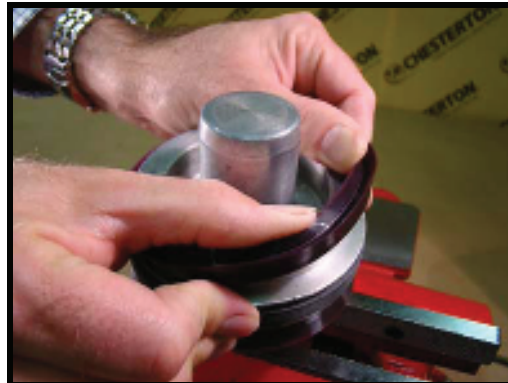
2. Hold piston securely, locate seal into groove and use finger pressure to begin stretching over piston head.
