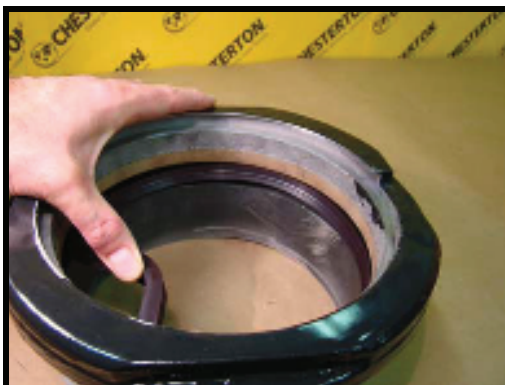
3. Push seal down and towards center of the gland. Release force and allow seal to snap into groove.
