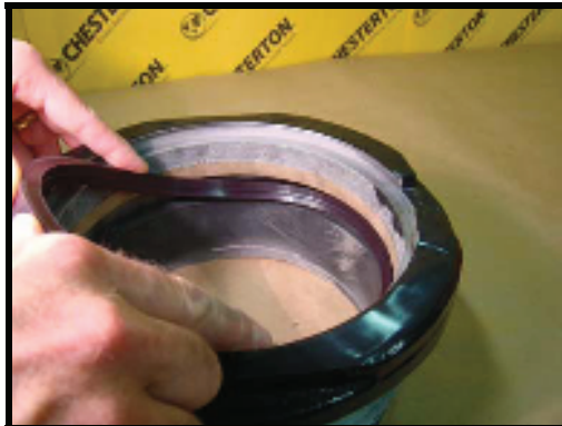
2. Locate the seal into the groove.
